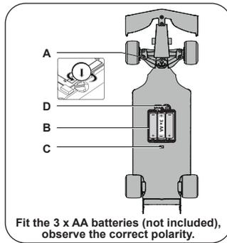
Fit the 3 x AA batteries (not included), observe the correct polarity.
